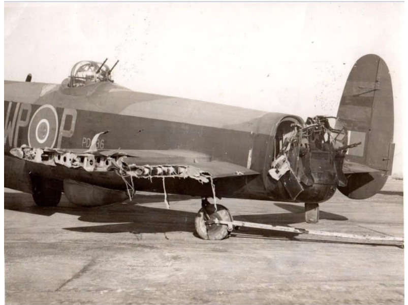
What I believe to be ground collision damage to PD336 WP-P
